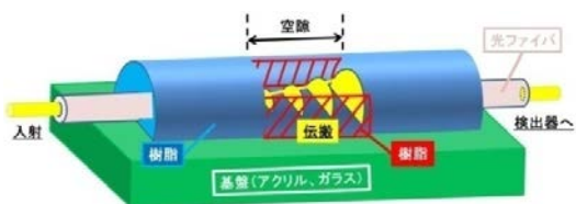
Fig. 2 Waveguide sensor using gapped fiber.
